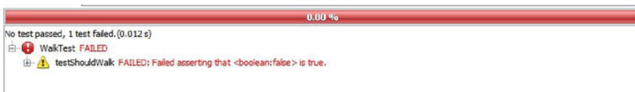
Figure 13-2. Netbeans IDE displaying a unit test failure
